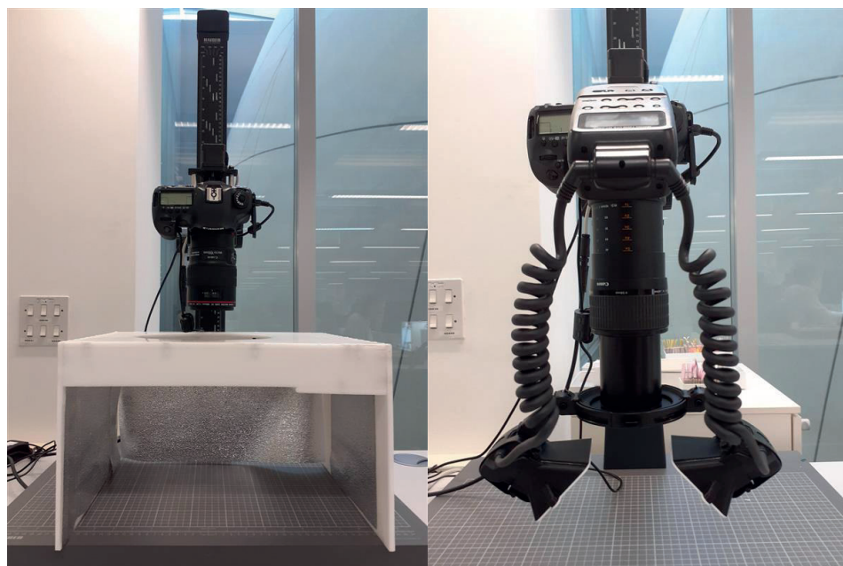
Figure 2. Imaging setup used for (left) overview and (right) stacked specimen photography.
